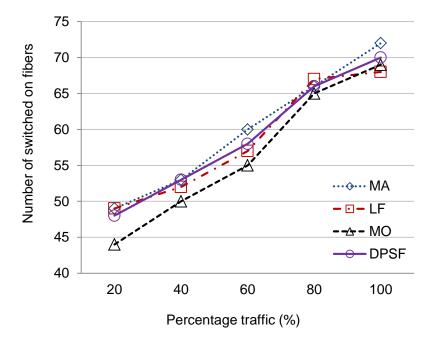
Figure 4.7: The number of switched-on fibers remaining against traffic variations
