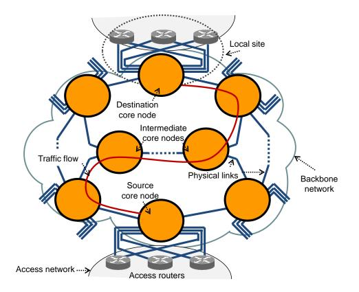
Figure 1.1: The fundamental architecture of a backbone network
