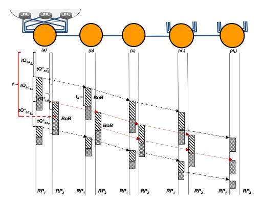
Figure 7.10: An example of an OBS network which accommodates traffic between node pairs  $(s, d_1)$  and  $(s, d_2)$  that arrives at a rate of  $R^{sd_1}$  and  $R^{sd_2}$ , respectively, using the **DPS burst assembly scheme**
