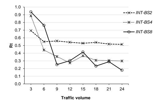
Figure 5.15: Power savings of a BSN using the **INT** grouping policy with respect to *different BS* and a **uniform** traffic model on the **NSF** network
