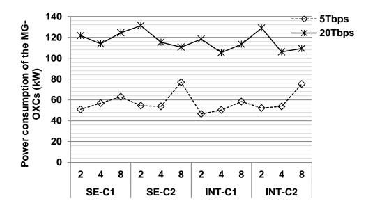
Figure 5.18: Power consumption of the MG-OXCs, using SE and INT grouping policies with C1 and C2 configurations, plotted against three band sizes
