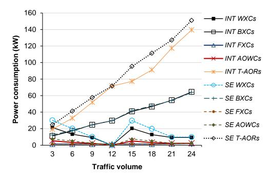
Figure 5.14: Device power consumption plotted against increasing traffic volume for each grouping policy on the **NSF** network, using a **uniform** traffic model
