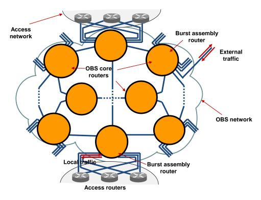
Figure 7.1: The fundamental architecture of an OBS network
