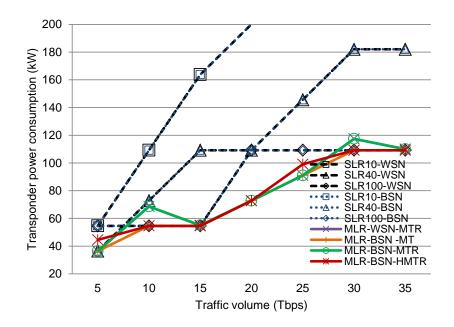
Figure 6.6: Power consumption of transponders at every traffic volume (Tbps) in all test networks
