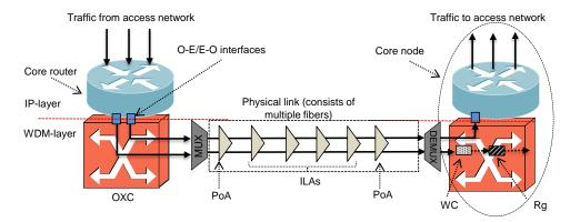
Figure 2.1: Constituent devices of an optical backbone network
