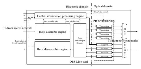
(b) Block diagram of an OBS line card [194]
