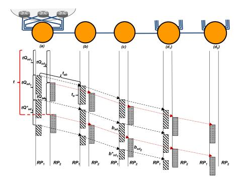
Figure 7.9: An example of a *traditional* OBS network which accommodates traffic between node pairs  $(s, d_1)$  and  $(s, d_2)$  that arrives at a rate of  $R^{sd_1}$  and  $R^{sd_2}$ , respectively, using the **DEB burst assembly scheme**
