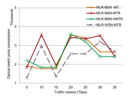
Figure 6.10: Number of optical switch ports consumed by MLR-based networks at every traffic volume (Tbps)
