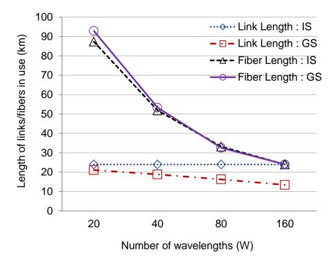
Figure 4.4: Total length of the fibers/links against increasing *W*.
