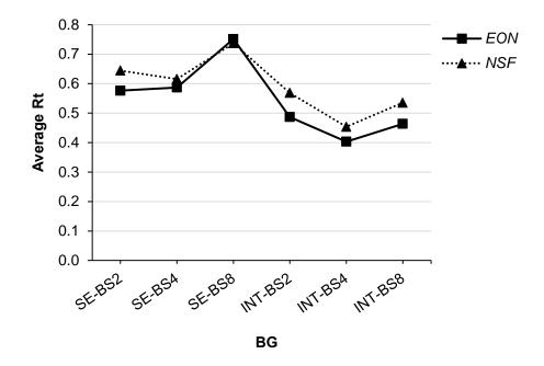
Figure 5.10: *Rt*, averaged over the range of traffic volumes distributed using the **uniform** traffic model, plotted against every BG on the **NSF** and **EON** networks
