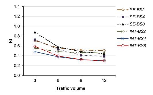
Figure 5.9: *Rt*, obtained for different BG on the **EON** network with a **gravity** traffic model, plotted against increasing traffic volume
