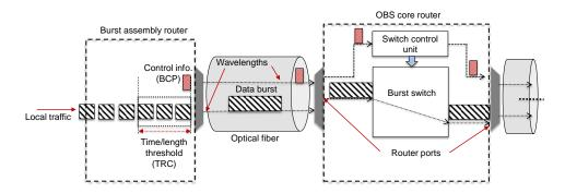
Figure 7.2: Key devices and operations of a burst assembly router and an OBS core router
