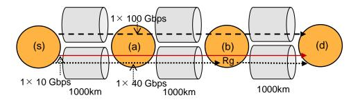
Figure 6.4: Assignment of rates for  $t^{sd}$  of 150 Gbps using the HMTR algorithm
