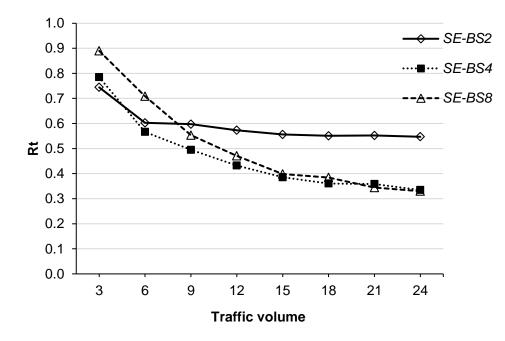
Figure 5.16: Power savings of a BSN using the **SE** grouping policy with respect to *different BS* and a **gravity** traffic model on the **NSF** network
