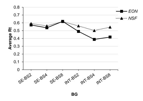
Figure 5.11: *Rt*, averaged over the range of traffic volumes distributed using the **gravity** traffic model, plotted against every BG in the **EON** and **NSF networks**
