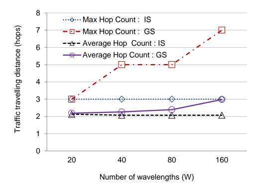
Figure 4.5: Number of hops travelled by traffic demands against increasing *W*.
