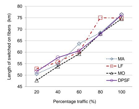
Figure 4.8: The total length of switched-on fibers remaining against traffic variations
