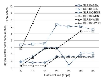
Figure 6.9: Number of optical switch ports consumed by SLR-based networks at every traffic volume (Tbps)
