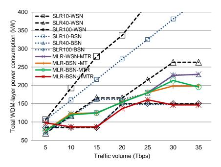
Figure 6.12: Total power consumption of the WDM-layer devices of all test networks at every traffic volume (Tbps)
