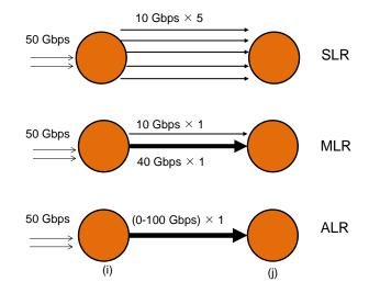
Figure 2.8: Rates assigned by SLR, MLR, and ALR techniques when transporting 50 Gbps of traffic from node i to j.
