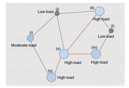
Figure 2.7: A backbone network using load-adaptive techniques: The size of the circles are proportional to their capacity and line rates; the dotted and solid lines indicate light- and heavyloaded links, respectively.
