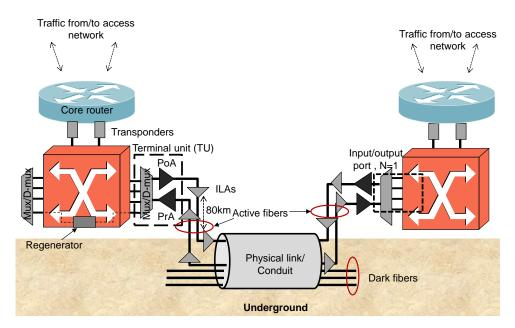
Figure 4.1: General architecture of the backbone network
