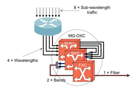
Figure 2.5: Aggregating traffic at multiple granularities by an MG-OXC of a Band Switched Network (BSN)
