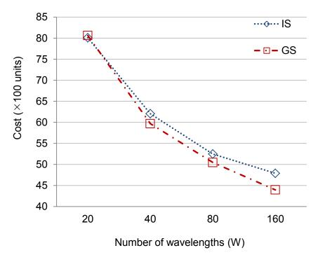
Figure 4.2: CAPEX against increasing W
