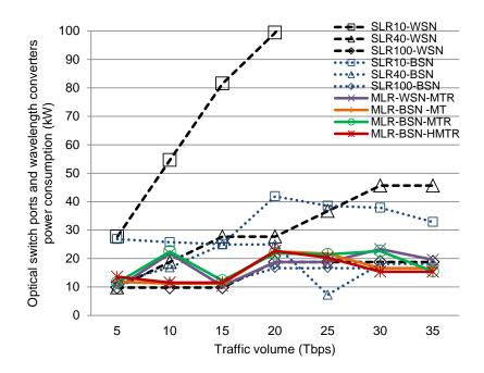
Figure 6.11: Combined power consumption of *optical switch ports* and *wavelength converters* at every traffic volume (Tbps) in all test networks
