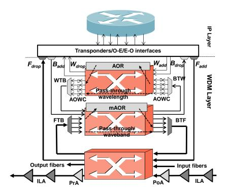
Figure 5.2: The architecture of a three-layer MG-OXC containing AOWCs and AORs
