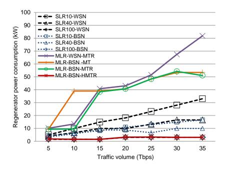
Figure 6.7: Power consumption of regenerators at every traffic volume (Tbps) in all test networks
