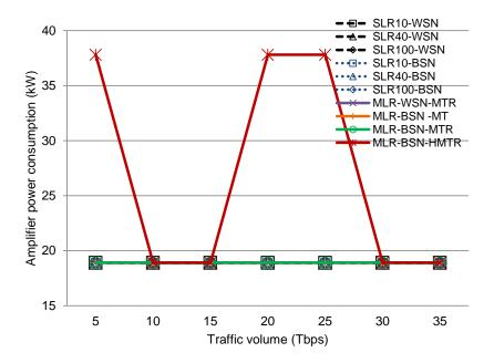
Figure 6.8: Power consumption of optical amplifiers at every traffic volume (Tbps) in all test networks
