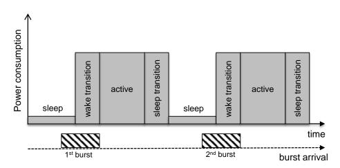
Figure 7.3: Power consumption at different operating states of a device in a sleep-mode-enabled OBS network
