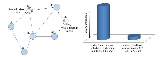
Figure 2.6: Switching nodes into sleep mode to reduce power consumption.
