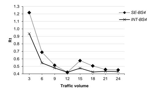
Figure 5.12: *Rt* of combinations *SE-BS4* and *INT-BS4* plotted against increasing traffic volumes on the **NSF** network using the **uniform** traffic model
