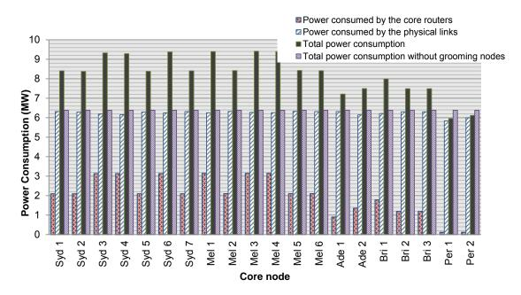
Figure 3.8: Power consumed by the core routers and physical (WDM) links with different grooming nodes
