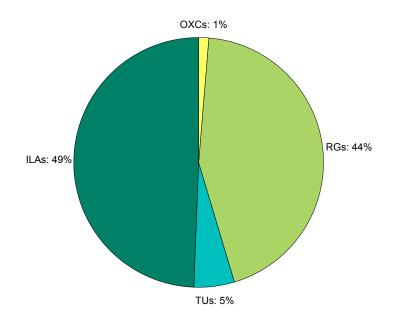
Figure 4.11: Percentage power consumption of network devices using the MO algorithm with peak-hour traffic)
