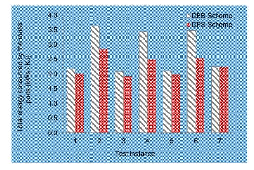
Figure 7.11: Power consumption of the router ports at every test instance when bursts are generated with the DEB and DPS schemes
