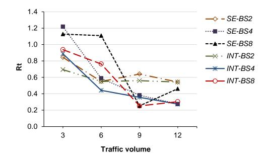
Figure 5.6: *Rt*, obtained for different combinations of band size and grouping policy (i.e., BG) on the **NSF** network with a **uniform** traffic model, plotted against increasing traffic volume
