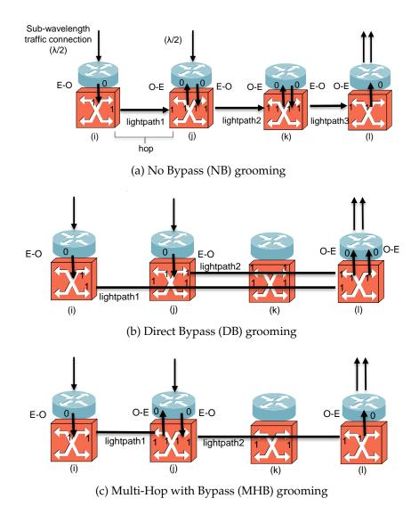
Figure 2.4: Comparison of the three wavelength grooming schemes
