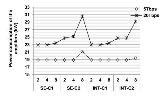
Figure 5.19: Power consumption of the amplifiers, using SE and INT grouping policies with C1 and C2 configurations, plotted against three band sizes
