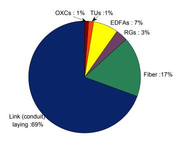
Figure 4.10: Breakdown of CAPEX
