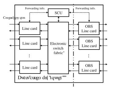
(a) Block diagram of a burst assembly router [194]
