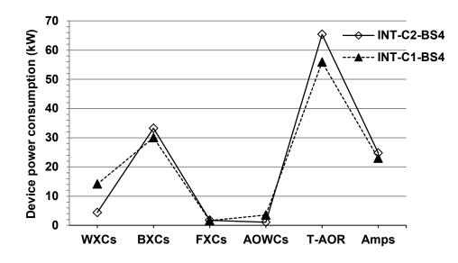
Figure 5.20: Power consumed by amplifiers and the individual devices of MG-OXCs, using C1 and C2 configurations with INT grouping policy and BS = 4, when total network traffic is 25 Tbps.
