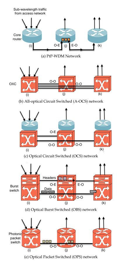
Figure 2.2: Different core node architectures
