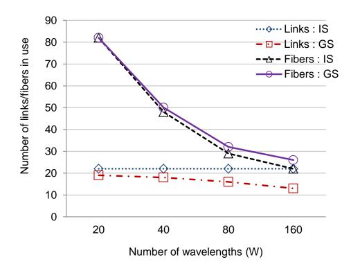
Figure 4.3: Number of fibers/links against increasing *W*.
