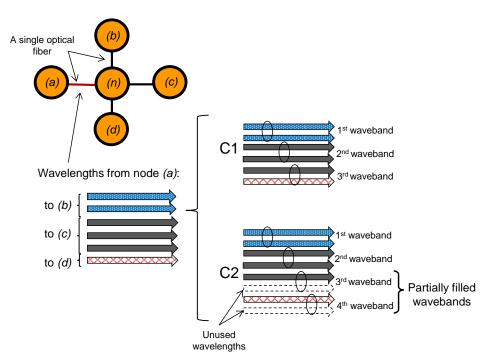
Figure 5.1: Comparison of C1 and C2 configurations with a uniform BS of 2
