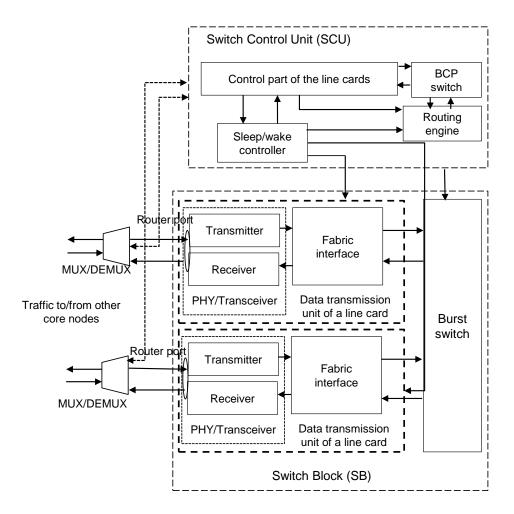
Figure 7.5: Block diagram of an OBS core router [120]
