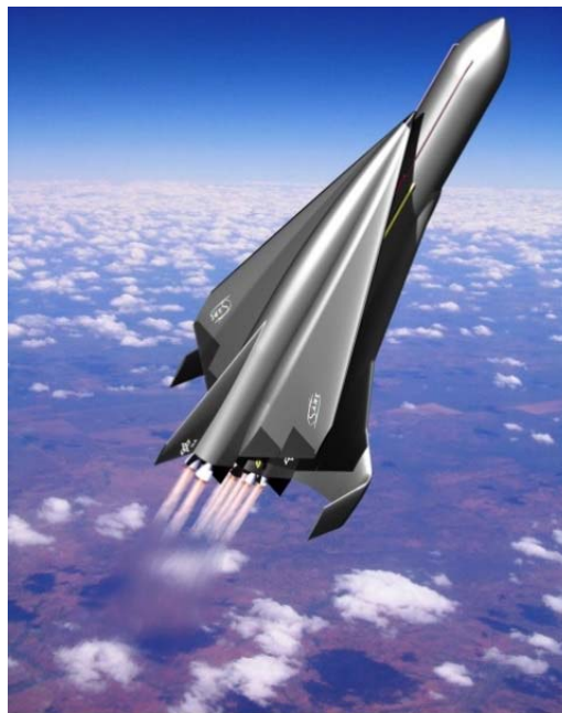
Figure 10: Visual representation of the latest SpaceLiner 7 launch configuration with passenger stage (top) and booster stage (bottom) with stage attachment [183]
