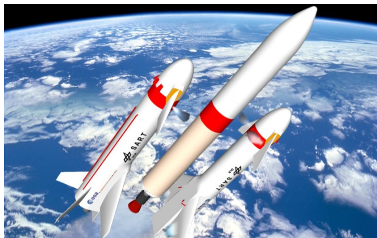
Figure 23: ASSC2-Y9 concept of a semi-reusable launch vehicle with A5 core stage and two attached, reusable fly-back boosters [46]
