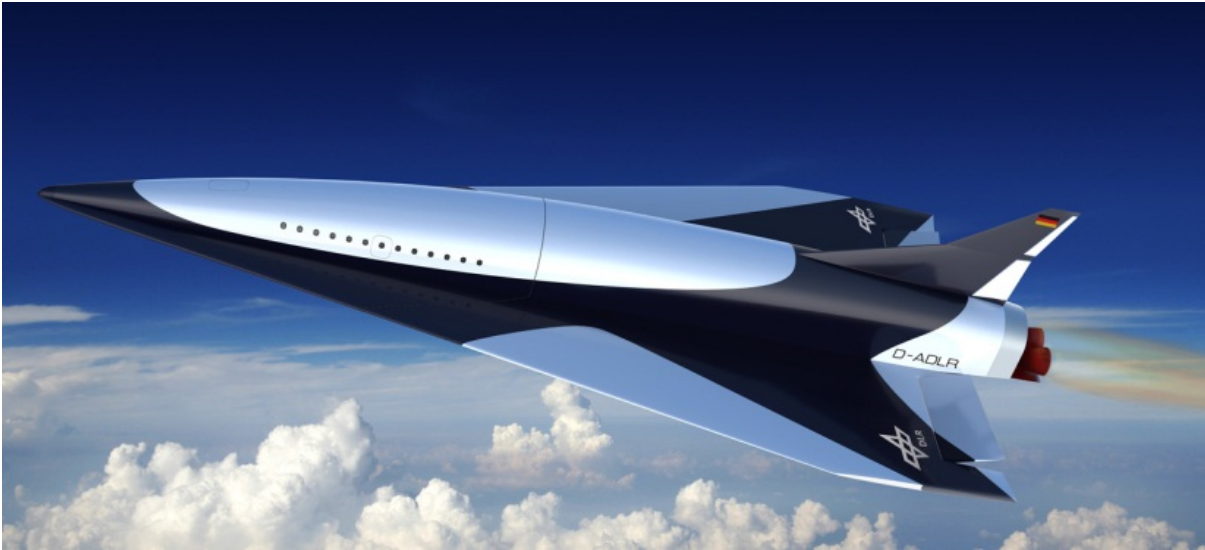
Figure 8: The SpaceLiner vision of an ultra-fast, rocket-propelled intercontinental, point-to-point passenger transportation spaceplane [82]
