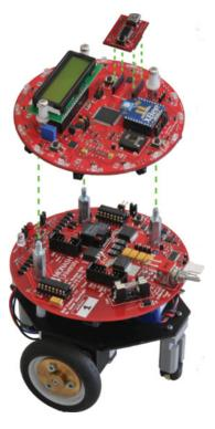
Fig. 6. Experimental robot eBug. It has a diameter of 120 mm and is equipped with two stepper motors driving two wheels independently. Further details about its hardware and firmware can be found in.<sup>13</sup>
